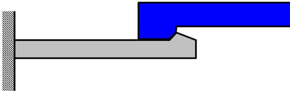
**Figure 2. A snap fastener and its mating lug**
