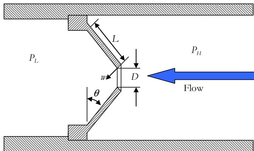
As the flow rate through the valve increases, the pressure differential across the diaphragm increases. The diaphragm then deflects under the uniform load, and the orifice diameter  $D$  reduces. This reduction increases the orifice coefficient, and the flow reduces back to its original value.
